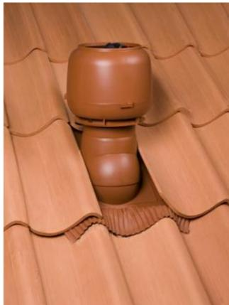
**ENG:** Then set all the tiles into place. You may have to cut off a piece from the bottom of some tiles, so that the tile sits evenly against the batten. Check with a builder's level that the pipe is vertical. Mount the pipes to the pass-through with six screws.
